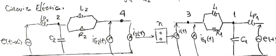
$$\text{Nº1: } V_1 \left( C_1 D + \frac{1}{R_1} + \frac{1}{L_1 D} + \frac{1}{L_{p1} D} \right) - E(t) \cdot \frac{1}{L_{p1} D} - V_3 \left( \frac{1}{R_1} + \frac{1}{L_1 D} \right) = 0$$
