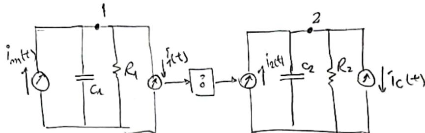
$$\text{Nó 1: } V_1 \left( C_1 D + \frac{1}{R_1} \right) = i_m - i_1 \rightarrow \text{Nó 1: } W_1 (J_1 D + B_1) = T_m - T_1 \Rightarrow J_1 \ddot{\theta}_1 + B_1 \dot{\theta}_1 = T_m - T_1$$
