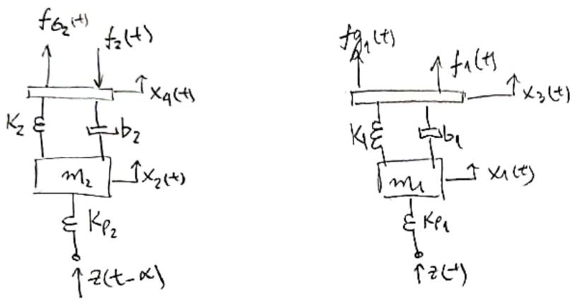
$$\left. \begin{array}{l} f_2(t) = l_2(K_2\theta + b_2\dot{\theta}) \\ f_1(t) = l_1(K_1\theta + b_1\dot{\theta}) \end{array} \right\} \text{ARFAGEM}$$
