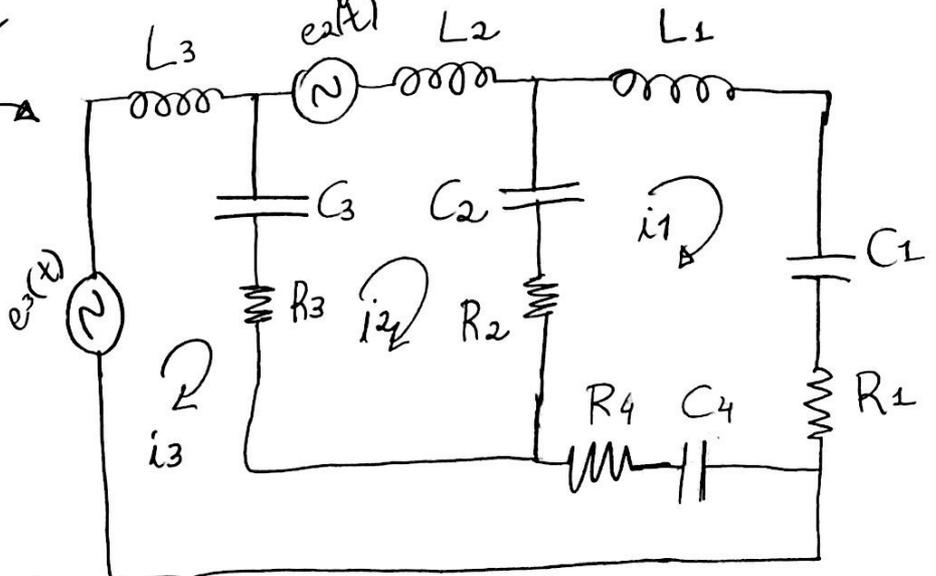
$$\begin{cases} e_3(t) = L_3 D i_3 + \left( R_3 + \frac{1}{C_3 D} \right) (i_3 - i_2) + \left( R_4 + \frac{1}{C_4 D} \right) (i_3 - i_1) \\ e_2(t) = L_2 D i_2 + \left( R_2 + \frac{1}{C_2 D} \right) (i_2 - i_1) + \left( R_3 + \frac{1}{C_3 D} \right) (i_2 - i_3) \\ \left( L_1 D + R_1 + \frac{1}{C_1 D} \right) i_1 + \left( R_2 + \frac{1}{C_2 D} \right) (i_1 - i_2) + \left( R_4 + \frac{1}{C_4 D} \right) (i_1 - i_3) = 0 \end{cases}$$
