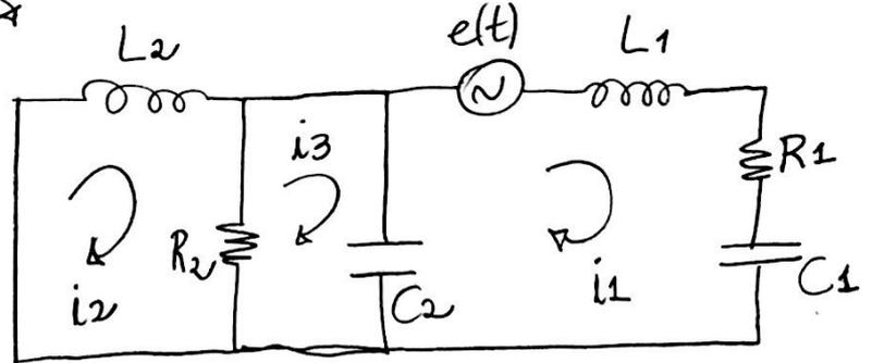
$$\left\{ \begin{aligned} \left( L_1 D + R_1 + \frac{1}{C_1 D} \right) i_1 + \frac{1}{C_2 D} (i_1 - i_3) &= e(t) \\ L_2 D i_2 + R_2 (i_2 - i_3) &= 0 \\ R_2 (i_3 - i_2) + \frac{1}{C_2 D} (i_3 - i_1) &= 0 \end{aligned} \right.$$
