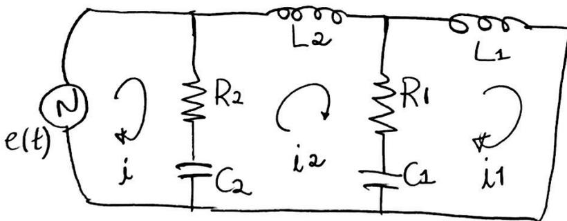
$$\left\{ \begin{array}{l} \left( R_2 + \frac{1}{C_2 D} \right) (i_1 - i_2) = e(t) \\ L_2 D i_2 + \left( R_1 + \frac{1}{C_1 D} \right) (i_2 - i_1) + \underbrace{\left( R_2 + \frac{1}{C_2 D} \right) (i_2 - i_1)}_{-e(t)} = 0 \\ L_1 D i_1 + \left( R_1 + \frac{1}{C_1 D} \right) (i_1 - i_2) = 0 \end{array} \right.$$
