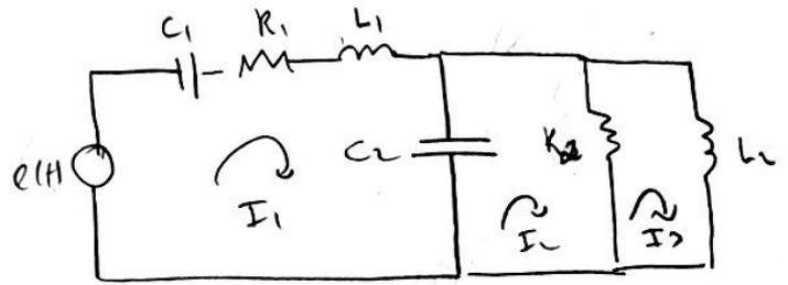
malha 1:  $C_1 \frac{1}{C_1 D} + R_1 I_1 + L_1 D I_1 + \frac{1}{C_2 D} (I_1 - I_2) = e(t)$
