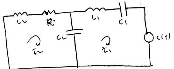
$$\text{malha 1: } L_2 D i_2 + \frac{1}{C_2 D} i_2 + \frac{1}{C_2 D} (i_2 - i_1) = e(t)$$
