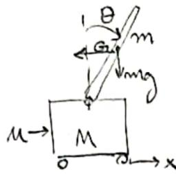
$$T_{BARRA} = \frac{1}{2}m\dot{x}^2 + m(\dot{x}\vec{v})[(-\dot{\theta}\vec{R}) \times l(\cos\theta\vec{j} + \sin\theta\vec{i})] + \frac{1}{2}(\dot{\theta})^2 \frac{4}{3}ml^2$$
