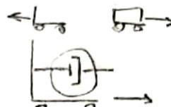
$$\begin{aligned} f_K &= K \cdot (x - y) \\ f_b &= b \cdot (\dot{x} - \dot{y}) \end{aligned}$$
