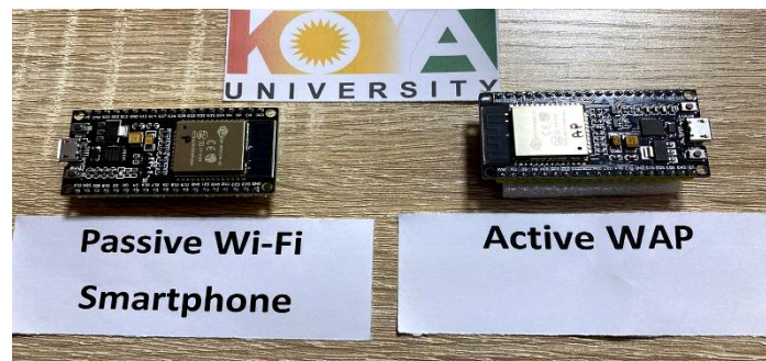
Figure 2: The two Wi-Fi EPS32 chipsets, left one is representing as a Smartphone, right one is working as WAP.
